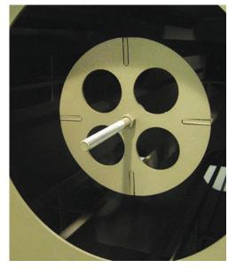
Structural steel cartridge supports self-center cartridges for easy removal and replacement.
