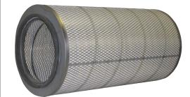
Each filter cartridge has 252 square feet of filter area with an efficiency rating of 99.7% for submicron (0.5) particulate.
